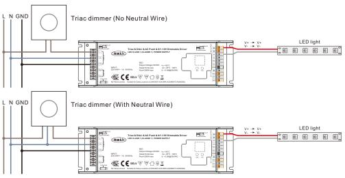
Note: After connecting the signal, you need to operate the control signal to dim 3-4 times (rotate the knob or long press the button to dim) to activate the current control signal.
